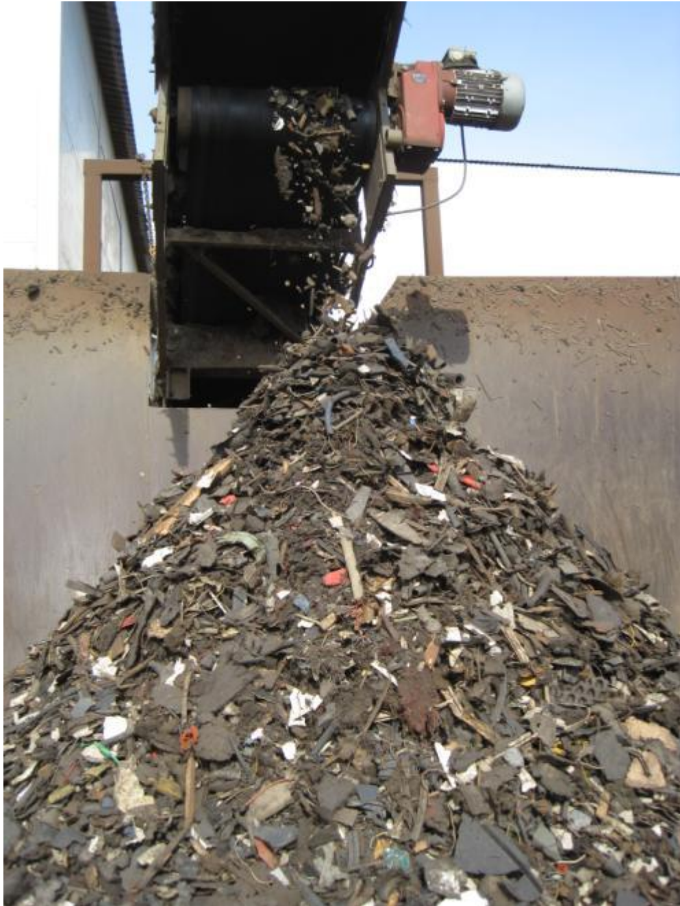
Figure 10: Rubber, Plastic, and Wood Fraction
