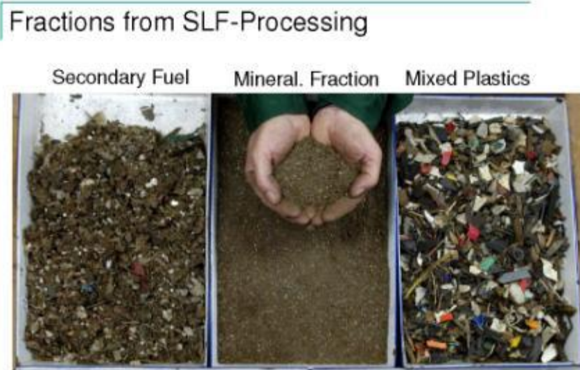
Figure 40: Fractions from Scholz SLF-Processing (Mehlhorn et al., 2009)
